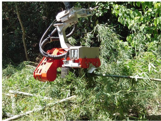
Figure 5. The harvesting head possesses a continuous processing function for clump bamboo logging.
