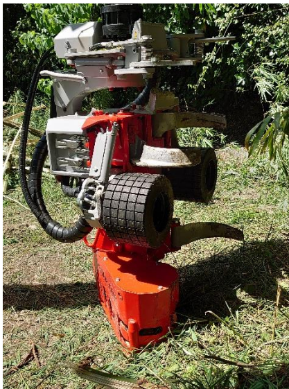
Figure 4. A pair of thick rubber replace original metal material on the feeding roller.
